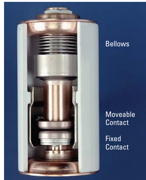
fig 3: principle vacuum interrupter
